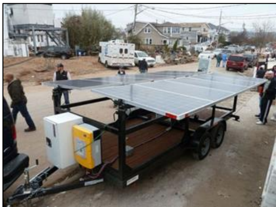
Figure 4: Solar generators used during Superstorm Sandy in New York [16]
