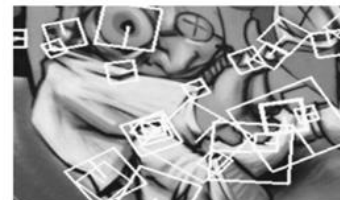
Fig5: Detail of the Graffiti scene showing the size of the oriented descriptor window at different scales
