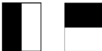
Fig3: Haar wavelet filters toward calculate the responses within x (left) as well as y direction (right). The shady parts contain the weight -1 along with the light parts +1
