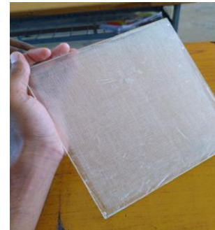
Fig 3.2 Fabricated composite laminates
