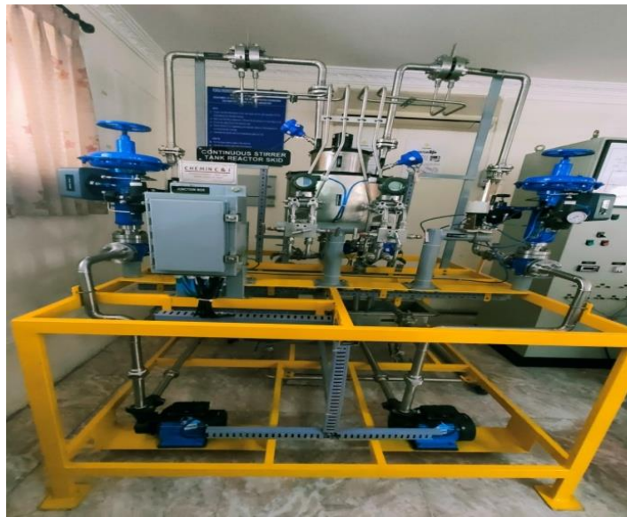
Fig- 2 Continuous Stirred Tank Reactor Skid
