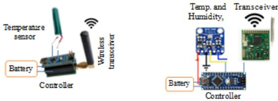
**Fig. 16(a)** Example on building wireless temperature module
