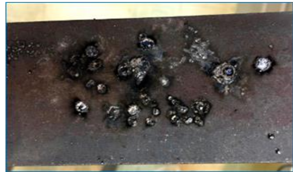
Figure (14): Barely spot weld produced when applying the weld on thicker low carbon steel with (5mm)
