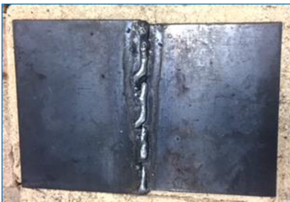
Figure (13): Short weld lines produced by using two transformers connected in parallel on low carbon steel with (2mm) thick
