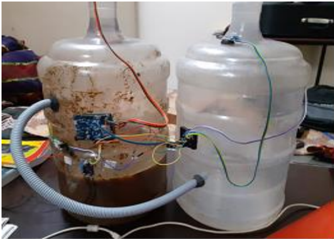
Figure 8. Hardware setup of Smart Sewage Monitoring System.
