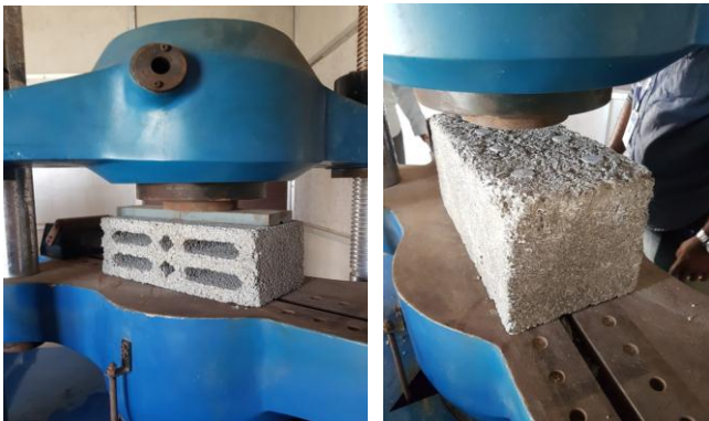
Fig 3. Testing of Concrete Hollow Block with and without plastic bottles
