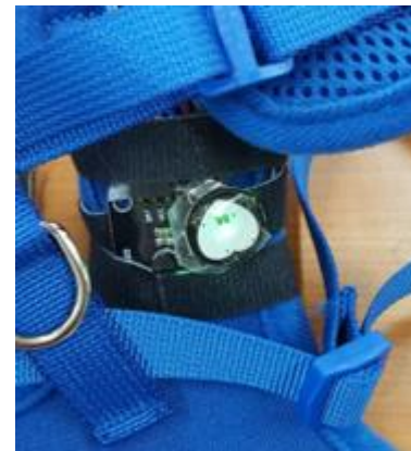
Fig. 3. IoT Device for data collections of ECG and temperature
