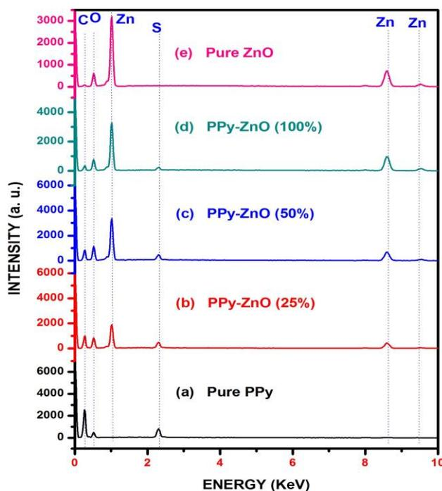
Fig.8 EDAX spectra of pure PPy (a), PPy-ZnO nanocomposites (b,c,d) and pure ZnO nPs (e)
