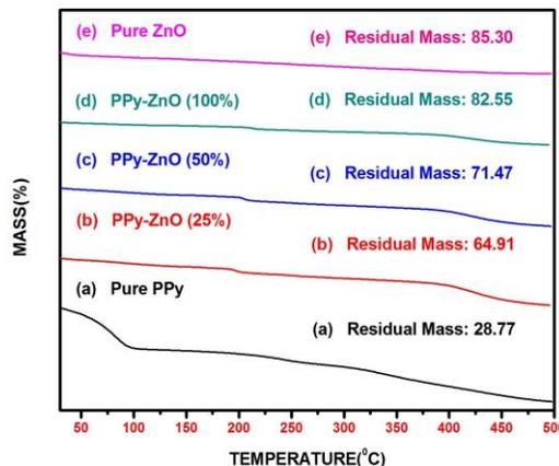
**Fig.5** TGA spectra of pure PPy (a), PPy-ZnO Nanocomposites (b, c, d) and pure ZnO nPs (e)
