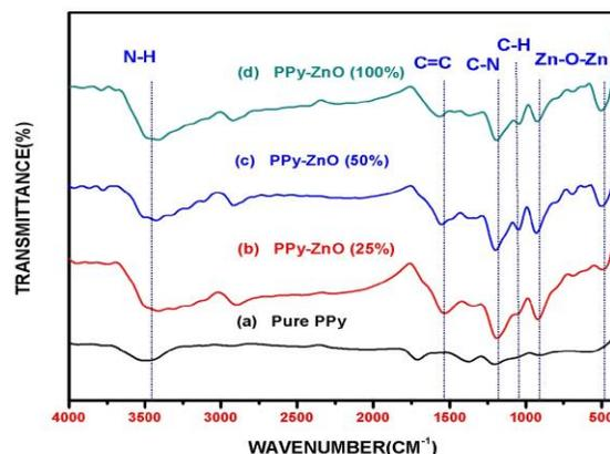
Fig.1 FTIR spectra of pure PPy (a) and PPy-ZnO nanocomposites (b, c & d)
