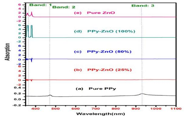
**Fig.2** UV-vis spectra of pure PPy (a), PPy-ZnO nanocomposites (b, c, d) and pure ZnO nPs (e)
