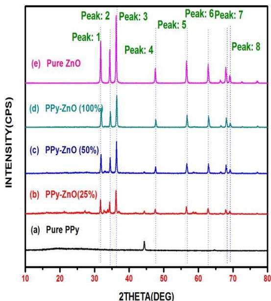
Fig.4 X-Ray diffraction patterns of pure PPy (a), PPy-ZnO nanocomposites (b, c, d) and pure ZnO nPs (e)
