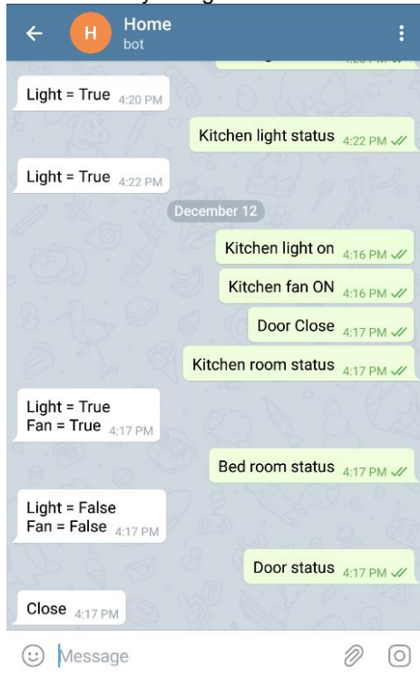
Fig. 12. Text Commands given in Telegram Bot to control HAS (Case 2)
