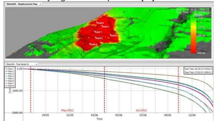
*Fig.6. A deformation plot and graph showing slope instability using SSR*
