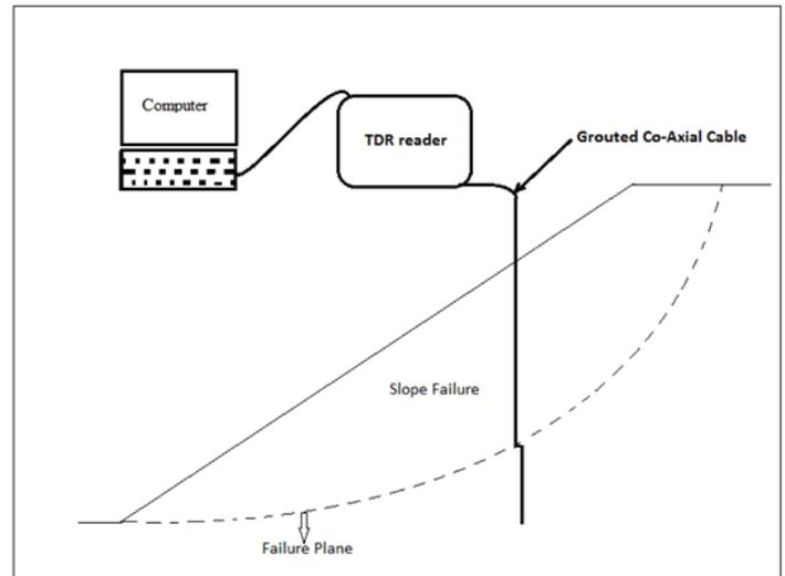
**Fig.2.** Working mechanism of TDR system
