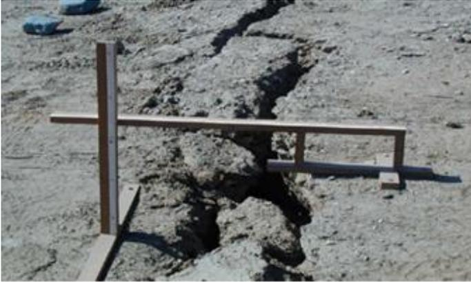
**Fig.3.** Device used as cross crack measurement after [7]
