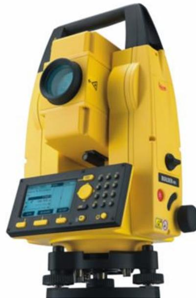
**Fig.4.** Total Station Monitoring Instrument
