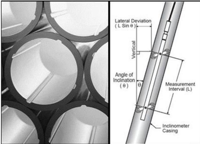
**Fig.1.** Groove inclinometer casing on the left and Inclinometer probe on the right
