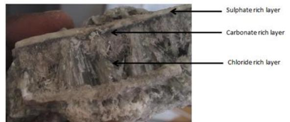
Figure 5 - Rock salt crust mined from the lake bed
