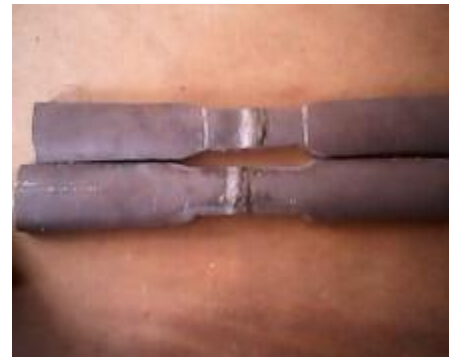
Fig. 3 Tensile Test samples before final preparation
