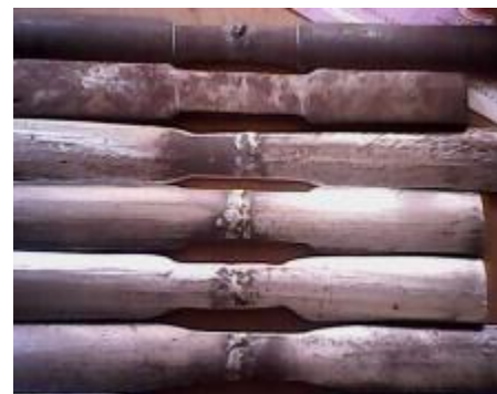
Fig. 4 Prepared samples for tensile tests
