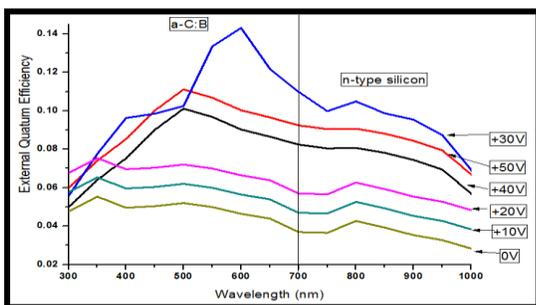
**Fig. 5. Spectral response of a-C:B solar cell fabricated with low positive bias voltage**
