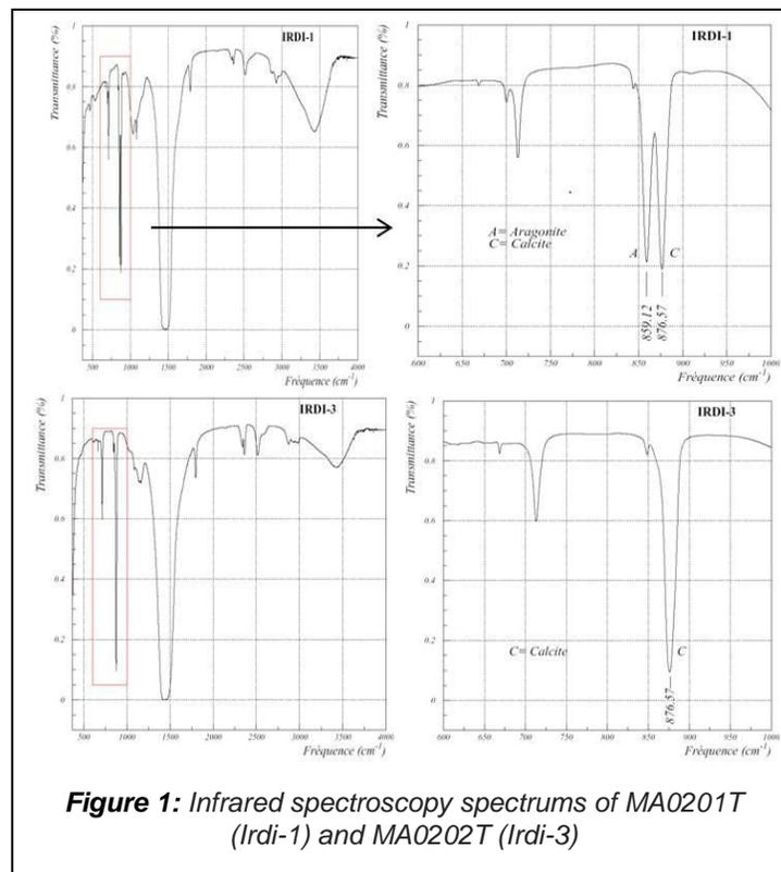
**Figure 1:** Infrared spectroscopy spectrums of MA0201T (Irdi-1) and MA0202T (Irdi-3)
