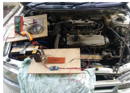
Figure 3: Experiment setup peltier for engine
