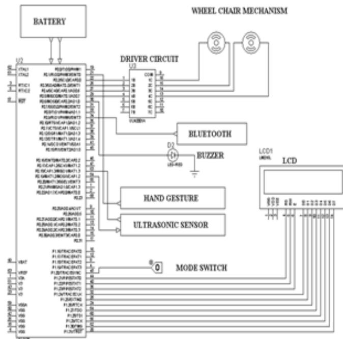
Fig.2 Circuit Diagram of the Proposed System
