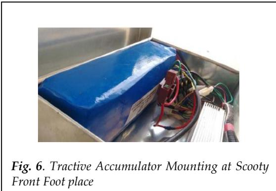
**Fig. 6.** Tractive Accumulator Mounting at Scooty Front Foot place
