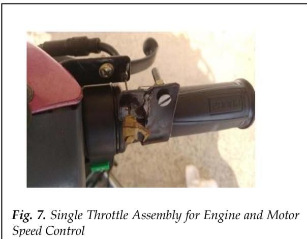
**Fig. 7.** Single Throttle Assembly for Engine and Motor Speed Control
