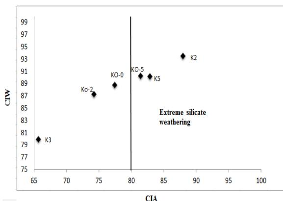
**Fig. 8.** Chemical index of alteration (CIA) versus chemical index of weathering (CIW) of Bensa kaolin plots area modified from N. N. Bukalo et al. [12]
