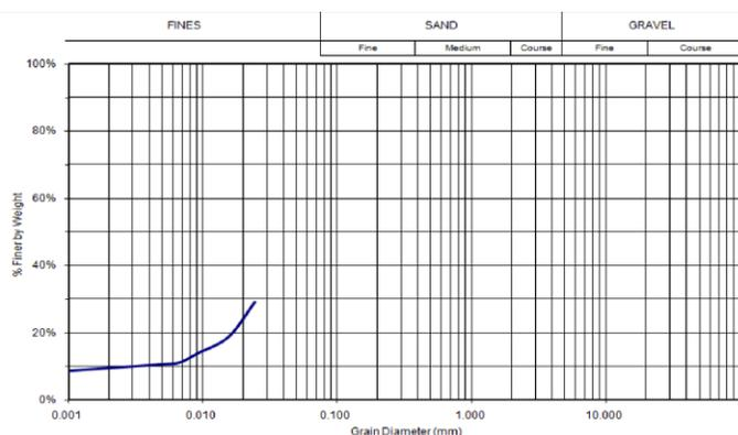
**Fig. 3.** Graph showing grain size analysis of Bensa kaolin sample from center of the deposit
