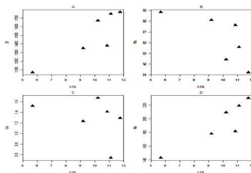
Fig. 6. Bensa kaolin samples trace element versus LOI variation diagram
