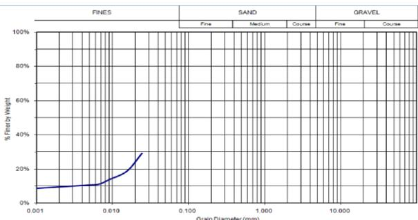
**Fig. 2.** Graph showing grain size analysis of kaolin samples from the periphery of the deposit
