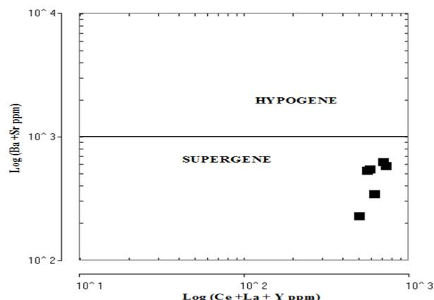
**Fig. 9.** Bensa kaolin samples on discrimination diagram of supergene-hypogene alteration of kaolin (fields are after H.G. Dill et al. [34])
