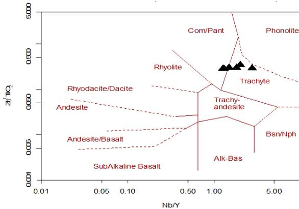
Fig. 4. Nb/Y Vs Zr/TiO<sub>2</sub> X 0.0001 plot after Winchester and [26] of Bensa and Koshe kaolin samples
