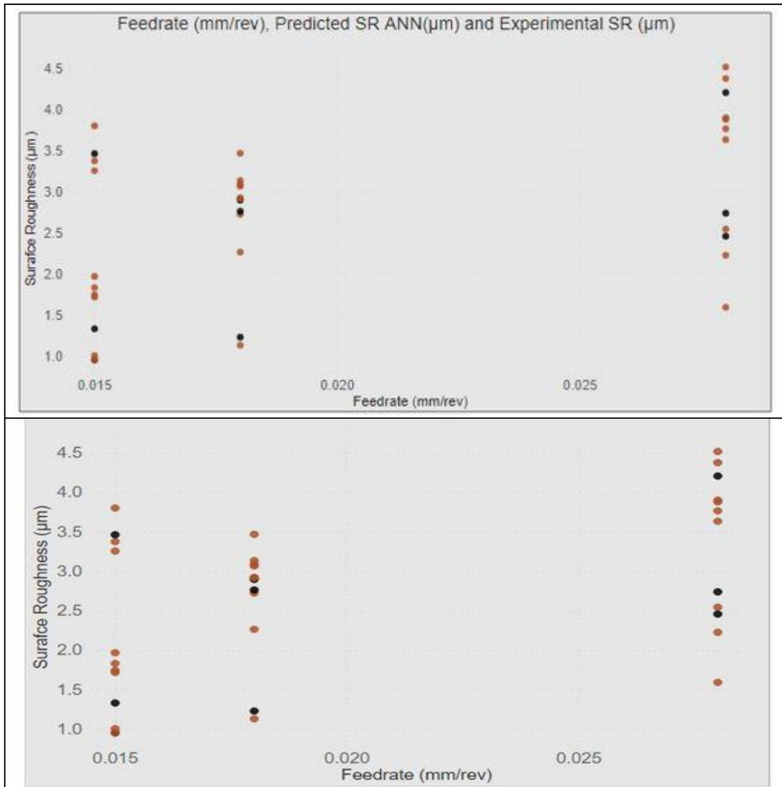
**Fig. 5 a) and b): Result of the experimental versus the predicted ANN**
