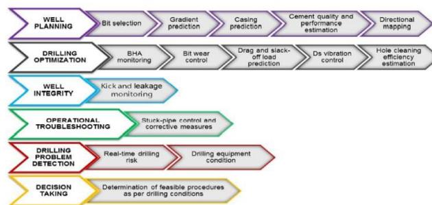
**Fig. 2: AI solutions for specific drilling processes and system design (Bello et al., 2016)**
