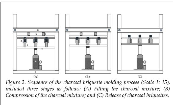
**Figure 2.** Sequence of the charcoal briquette molding process (Scale 1: 15), included three stages as follows: (A) Filling the charcoal mixture; (B) Compression of the charcoal mixture; and (C) Release of charcoal briquettes.
