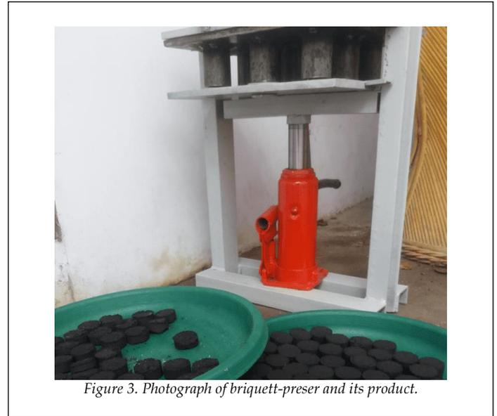
**Figure 3.** Photograph of briquet-presser and its product.
