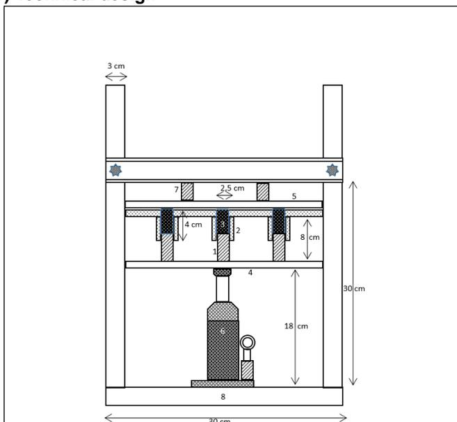
**Figure 1.** Technical specifications for charcoal briquette-presser (Scale 1:9). Description: (1) compression rod; (2) charcoal storage cylinder; (3) charcoal mix; (4) pressure plate; (5) top retaining
