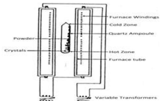
**Fig 1:** Schematic view of the furnace showing the position of ampoule inside the two zone furnace during crystal growth.
