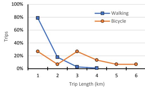
**Fig. 4: Trip Length Distribution for Non-Motorized Modes**
