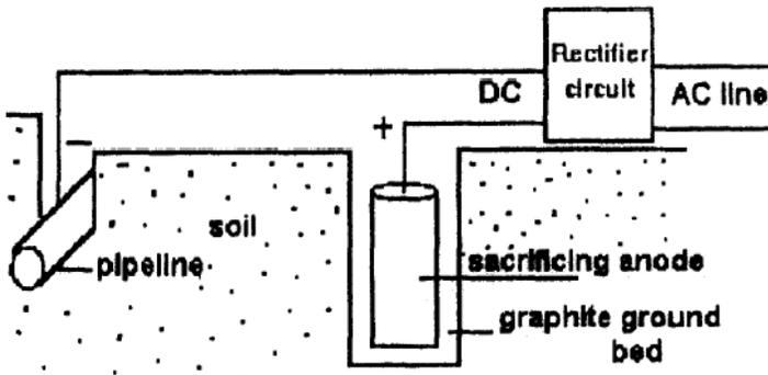
Fig1. Cathodically protected pipeline schematic diagram
