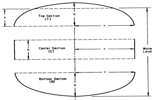
Fig 3.segmented elevated Tank for area calculations.
