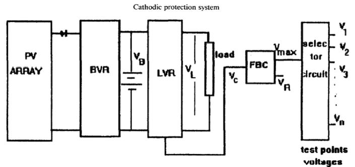
Fig2. Block diagram of the cathodic protection system
