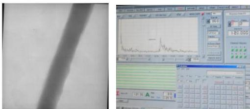
**Fig. 2. Images of a) radiographic, b) ultrasonic examinations of the weld zone on the study screen.**
