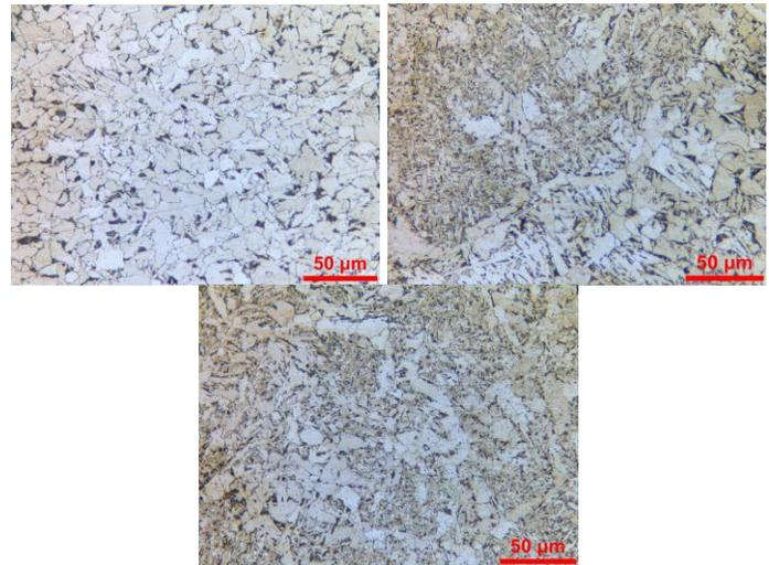
Fig. 6. Optical microscopic images of a) base metal, b) HAZ, and c) weld metal.
