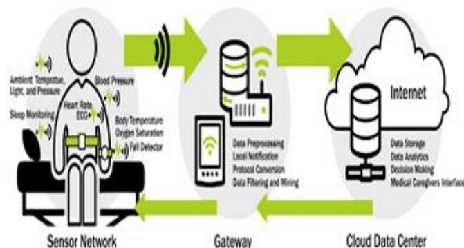
Fig. 2. General IoT-based health monitoring system [1]
