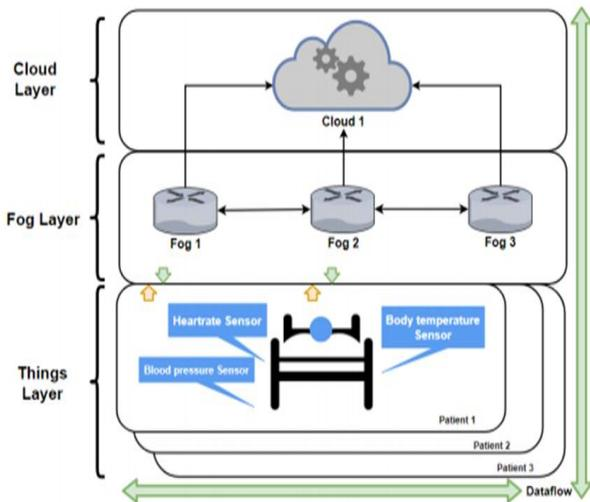
Fig. 7. IoT-Fog based Strata for Healthcare Systems [11]
