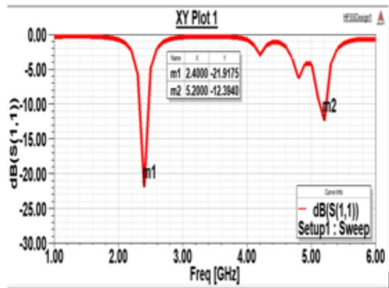
Fig. 4. Simulation result of the antenna
