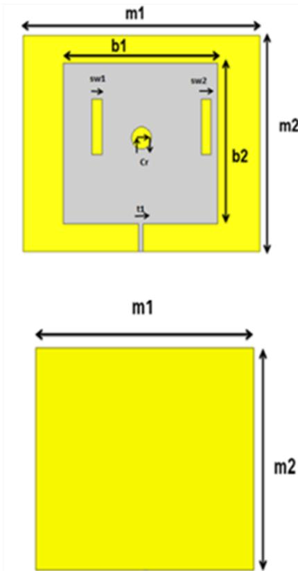
Fig. 2. Front and aback patch of the proposed antenna.
