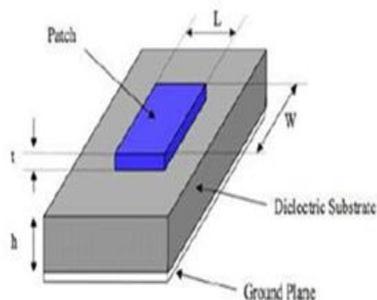
Fig 1: Illustration of a basic Microstrip patch antenna [9]
