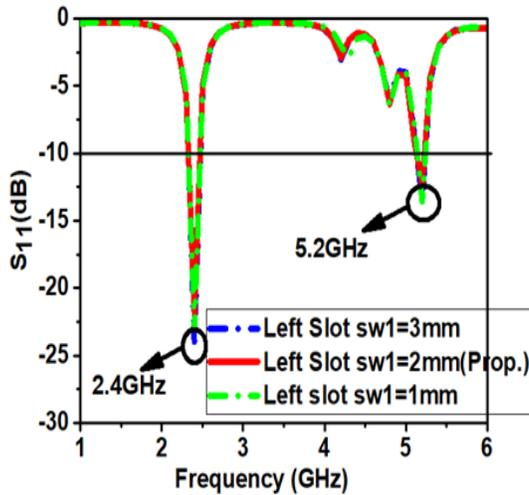
Fig. 3 (a). Effect of Slot sw1 on impedance matching of the antenna
