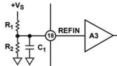
Fig. 3. Circuit diagram for internal reference
