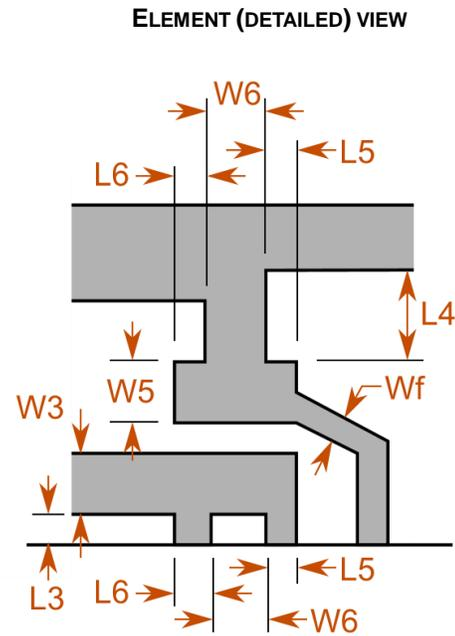
FIG.1. Top view, Side view, bottom view and elemental view of the antenna
