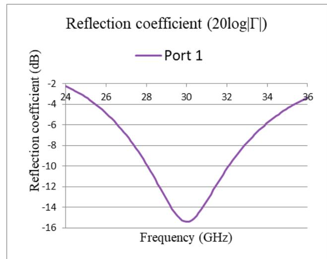
**Fig.3** Reflection Coefficient of the Antenna
