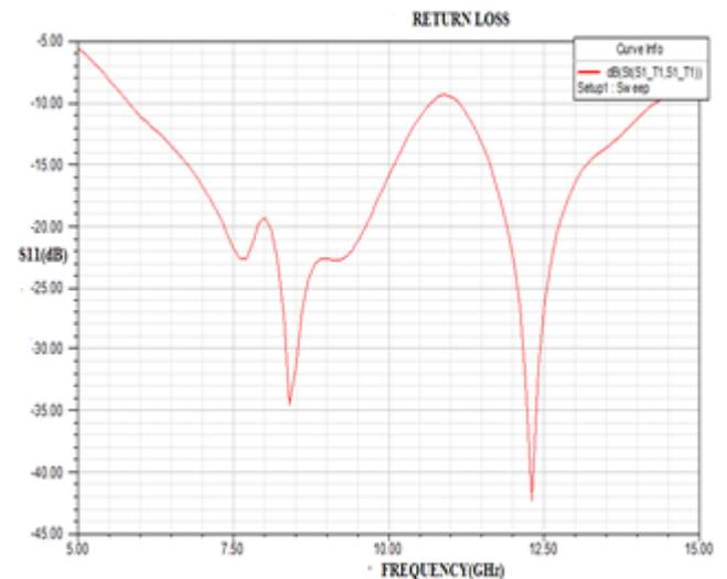
**Fig. 4. Impedance bandwidth of the antenna array**
