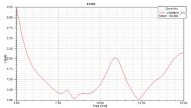
**Fig. 3. VSWR of the antenna array**
