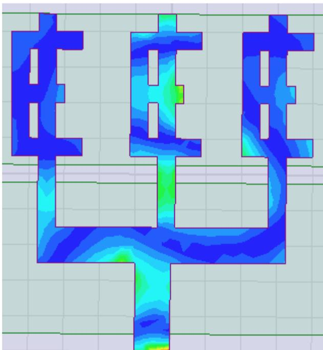
Fig. 5. Electric field representation of the antenna array
