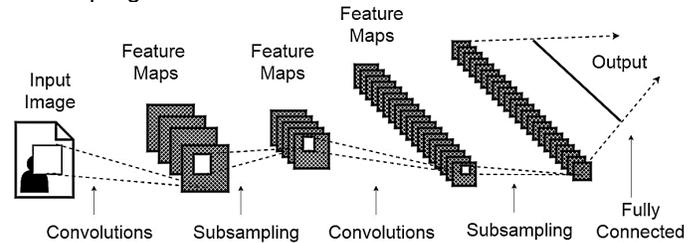
Fig. 2. Architecture of Convolution neural networks model
