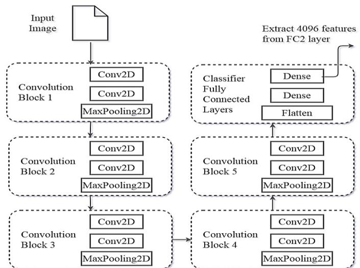
Fig. 3. Architecture of proposed VGG16 deep CNN model for feature extraction.
