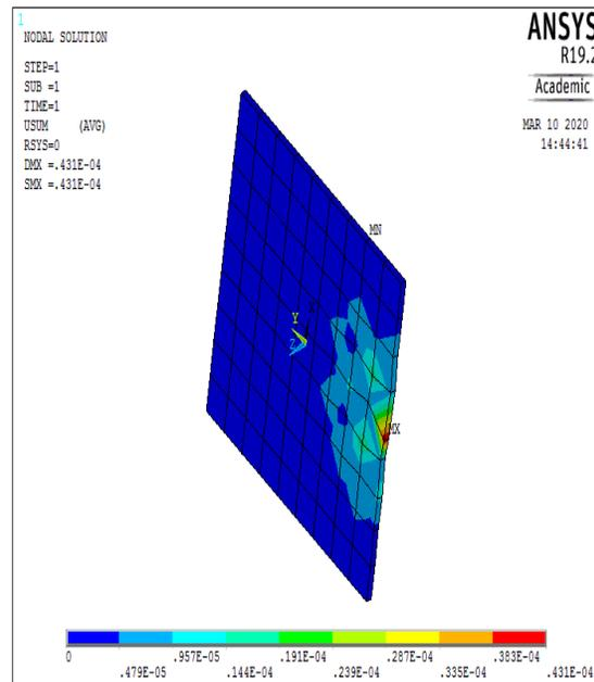
Figure 15 Displacement vector sum of Al 7075 alloy
