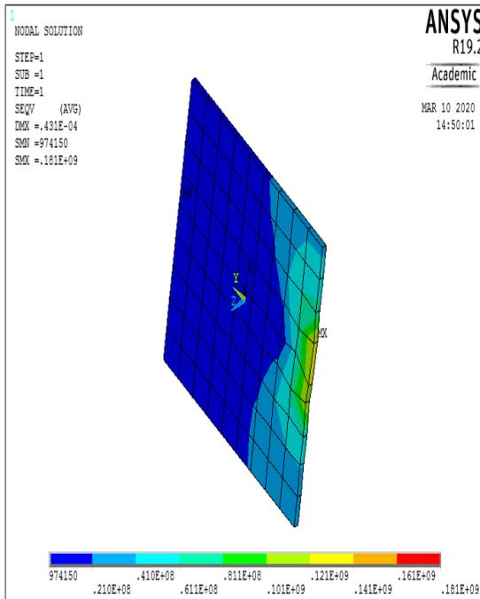
**Figure 16** Von mises stress of Al 7075 alloy
