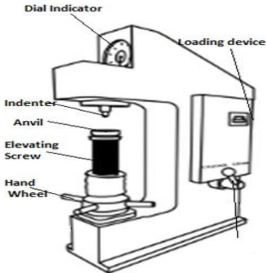
**Figure 12** Rockwell hardness tester
