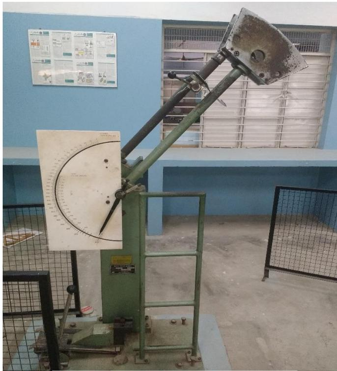
Figure 13 Experimental setup of Charpy test
