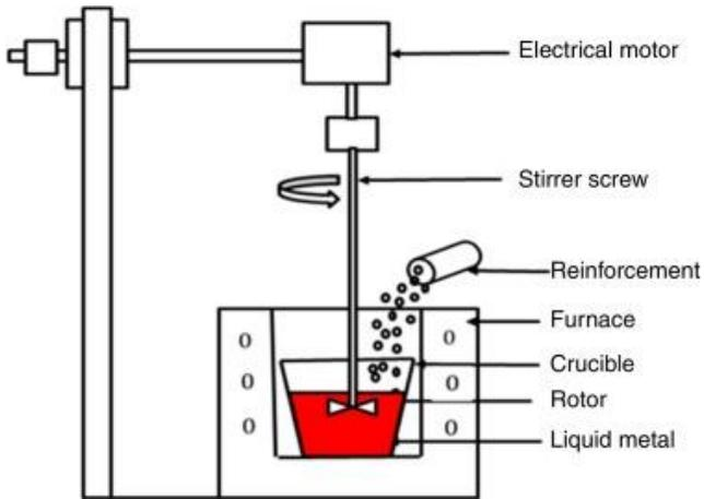
**Figure 2** Stir casting
