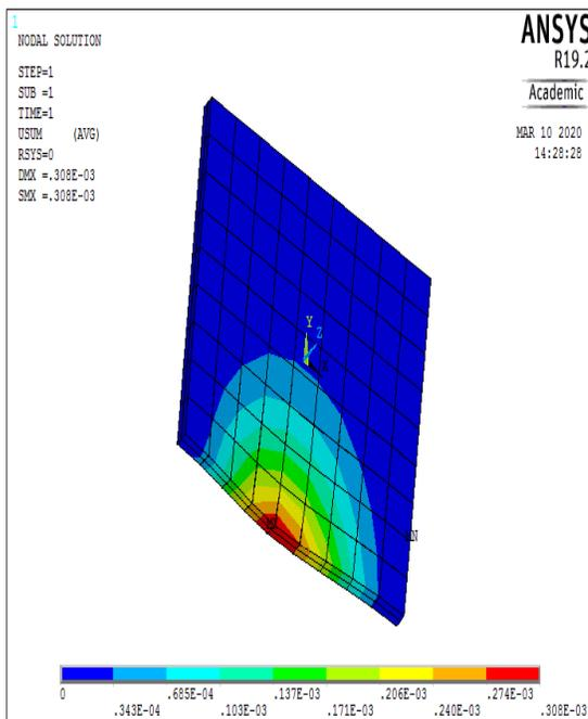
**Figure 17** Displacement Vector sum of Al 7075 and carbon nanotube composite
