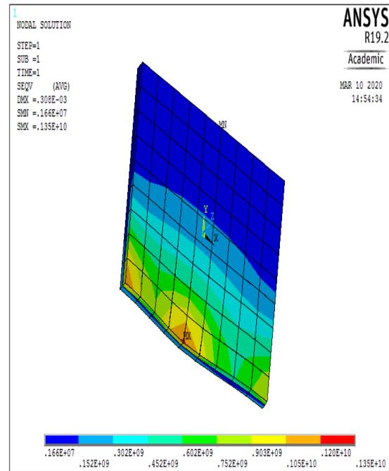
**Figure 18** Von mises stress of the Al 7075 and carbon nanotube composite
