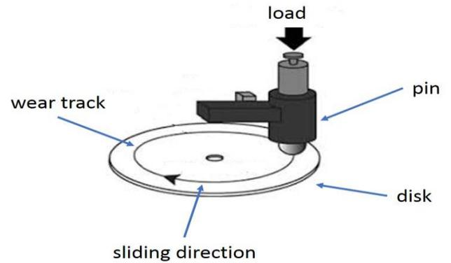
**Figure 3** Working of pin-on-disc tribometer.
