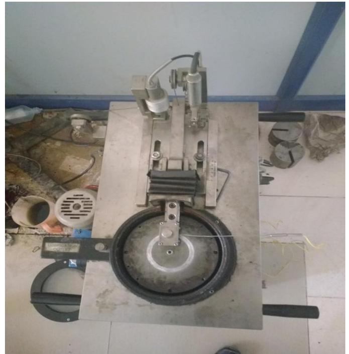
**Figure 4** Experimental setup of pin-on-disc tribometer
