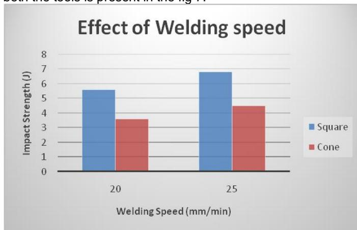
Fig 7. Effect of welding speed and pin profile on Impact strength
