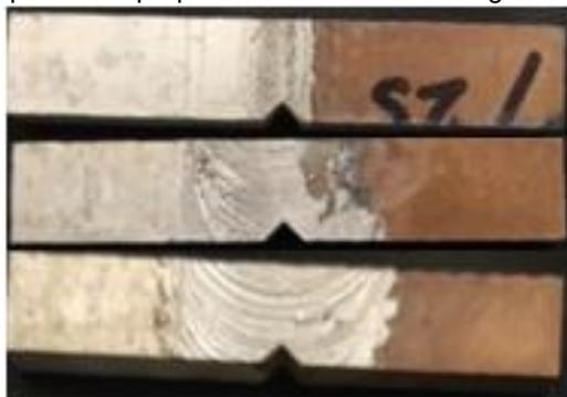
Fig 6. Izod Impact test sample specimen
