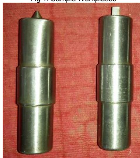
Fig 2. Cone and square pin FSW tool
