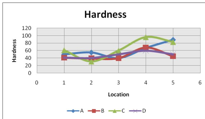
Fig 9. Hardness values in welded specimen
