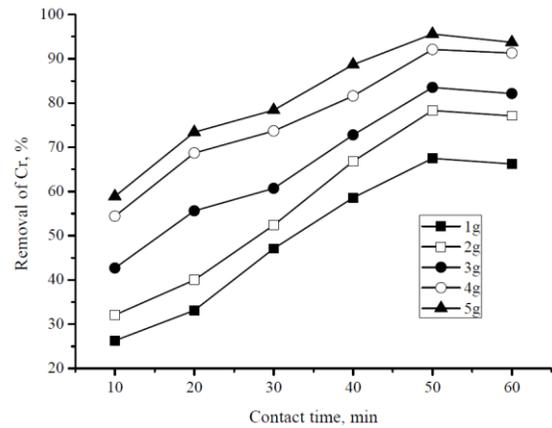
FIG 1 VARIATION OF %REMOVAL OF CHROMIUM AT VARIED CONTACT TIME FOR M1
