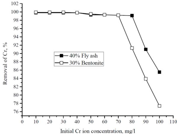
FIG 5 VARIATION OF %REMOVAL OF CHROMIUM AT VARIED INITIAL CONCENTRATION OF CHROMIUM AT OPTIMUM CONTACT TIME, PH AND ADSORBENT DOSAGE FOR BOTH M1 AND M2
