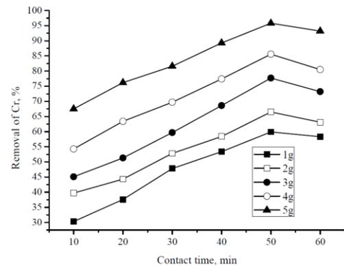
Fig 2 Variation of %removal of chromium at varied contact time for M2
