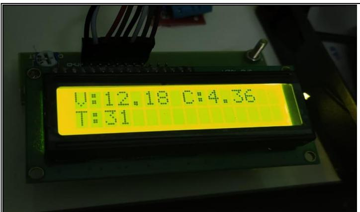
In Figure 4, the LCD is used to show the state of the transmission line, and enables the consumer to know the precise values of the sensor in real time. The monitor displays measurements of voltage in volts, current in ampere and temperature in celsius. In fact, this LED will also be used with the GPS module's latitude and longitude readings
