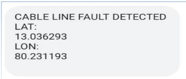
In Figure 9, when there happens a breakdown in the transmission line, the latitude and longitude of the affected point get recognized through the GPS module and these important points are sent as SMS to the approved cellular telephone thru the GSM module. The statistics is transferred via the air medium with the help of the GPS antenna.
