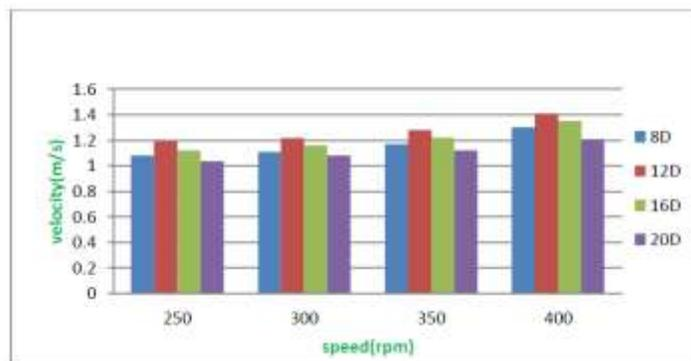
Figure.6 Velocity distribution of 3 wing ceiling fan
