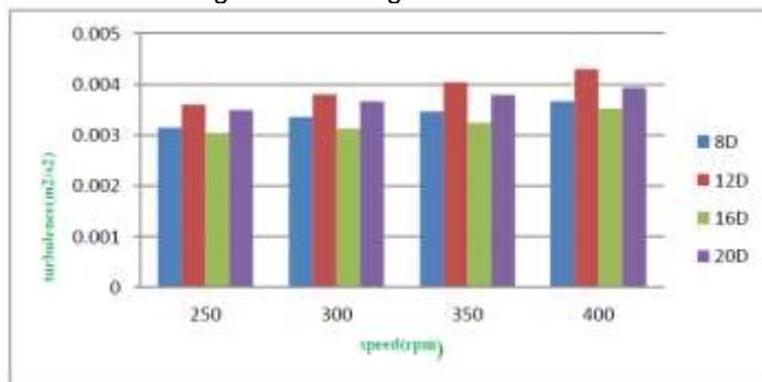
Figure.8 Turbulence kinetic energy distribution of 3wing fan
