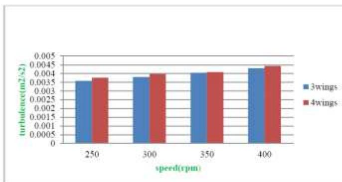
Figure. 10 Comparison of turbulence distribution of 3 winged and 4 winged fans
