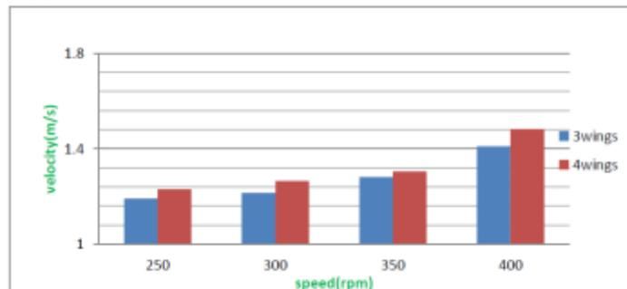
Figure.7 comparison of velocity distribution of 3 wings and 4 wings
