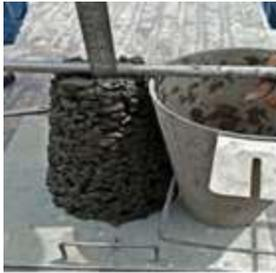
Fig. 1. Slump test of pervious concrete
