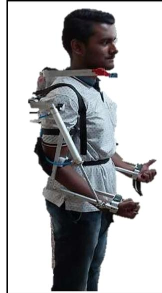
Figure 15. Basic Prototype of Exoskeleton
