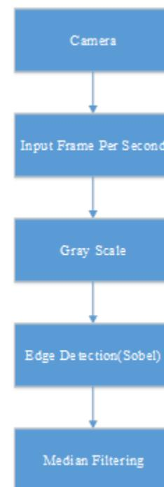
**Figure2.** Pre-Processing stage of traffic sign
