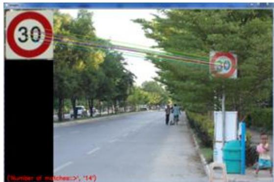
**Figure11:** Test result of speed limit road sign. This system work well with partial occlusion. The system should also be able to determine the exact speed limit, if the corresponding sign is classified as such.
