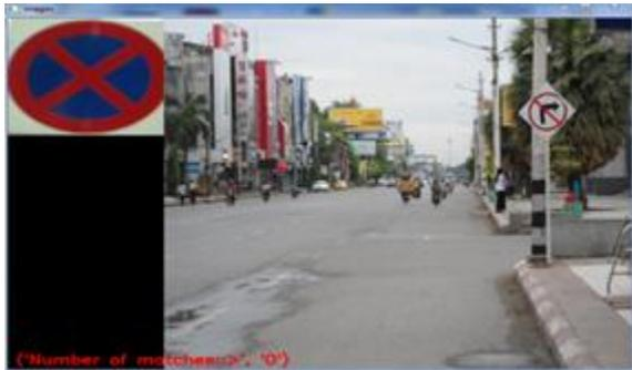
**Figure10:** Test result of no stopping road sign in database has no corresponding key points with no right turn road sign in original image
