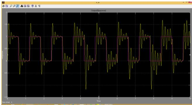
**Figure 8.** The simulation results of WNCS with 20 ms sampling rate
