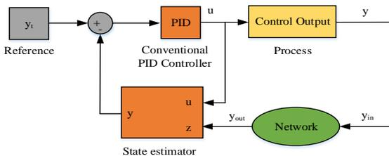
Figure 2. State estimator and regular PID controller for WNCs
