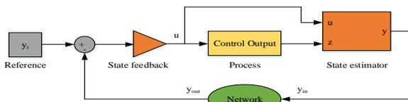
Figure 1. Optimal state feedback architecture for WNCs
