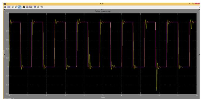
**Figure 7.** the simulation results of WNCS with 10ms sampling rate
