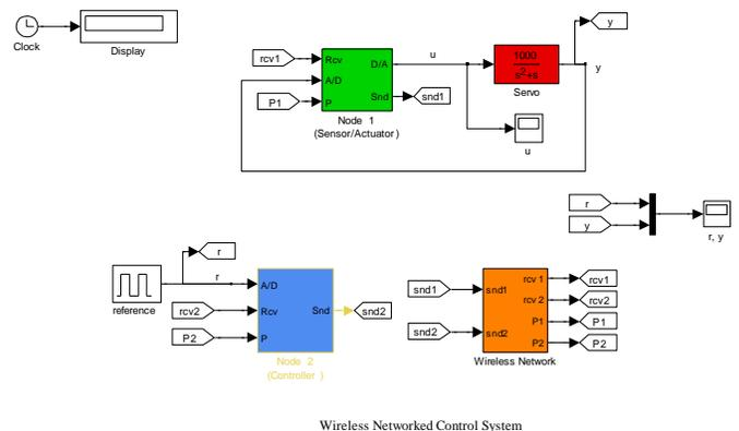
**Figure 6.** Simulink Model of Wireless Networked Control System
