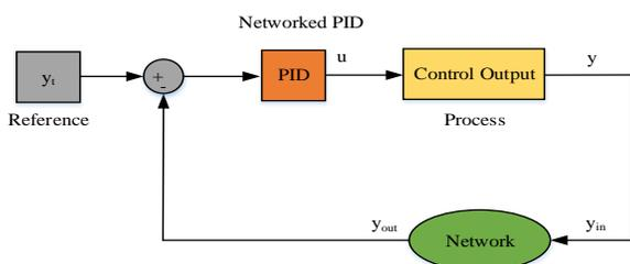
Figure 3. Jitter margin tuned PID controller for WNCs
