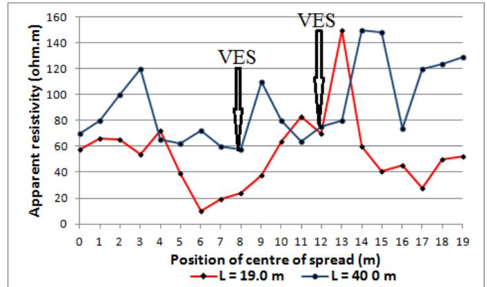
Fig. A5 Schlumberger resistivity profiles, showing apparent resistivity as a function of position of centre of spread for two values of electrode separation, Zei Community.
