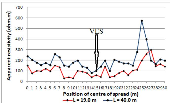
Fig. A10 Schlumberger resistivity profiles, showing apparent resistivity as a function of position of centre of spread for two values of electrode separation, Kanshegu Community.
