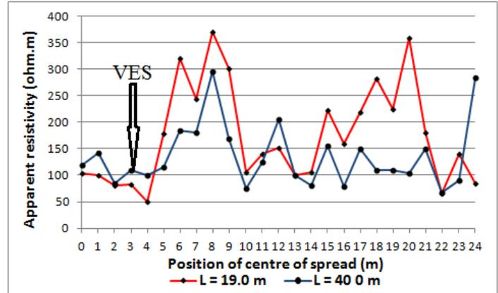
Fig. A6 Schlumberger resistivity profiles, showing apparent resistivity as a function of position of centre of spread for two values of electrode separation, Zei Community.
