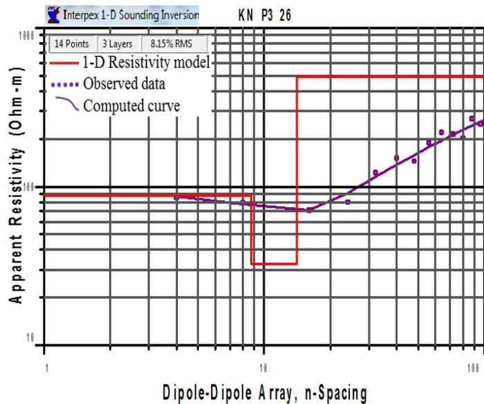
**Fig. 21** Iterated field curve and the apparent resistivity model of VES conducted at 260 m from the beginning of profile 3, Kanshegu Community (KN P3 26).
