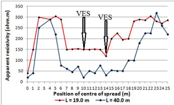
Fig. A8 Schlumberger resistivity profiles, showing apparent resistivity as a function of position of centre of spread for two values of electrode separation, Zantele Community.
