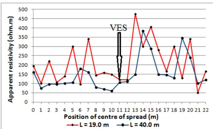
Fig. A4 Schlumberger resistivity profiles, showing apparent resistivity as a function of position of centre of spread for two values of electrode separation, Zei Community.
