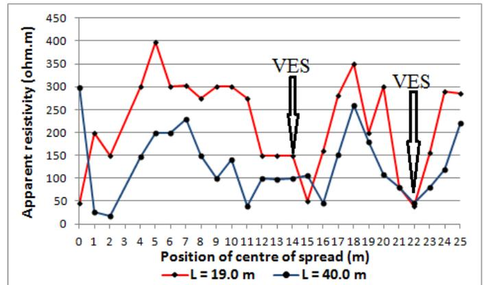
Fig. A7 Schlumberger resistivity profiles, showing apparent resistivity as a function of position of centre of spread for two values of electrode separation, Zantele Community.
