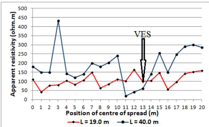
Fig. A3 Schlumberger resistivity profiles, showing apparent resistivity as a function of position of centre of spread for two values of electrode separation, Nyengbalo Community.
