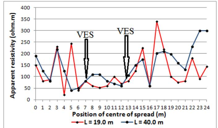
Fig. A11 Schlumberger resistivity profiles, showing apparent resistivity as a function of position of centre of spread for two values of electrode separation, Kanshegu Community.
