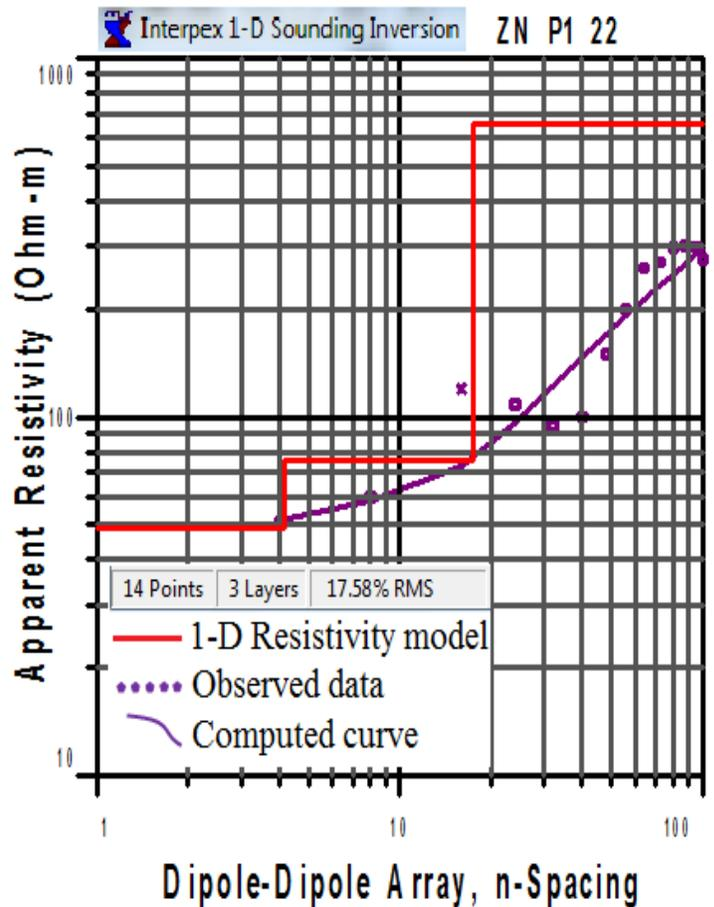
Fig. 12 Iterated field curve and the apparent resistivity model of VES conducted at 220 m from the beginning of profile 1, Zantele Community(ZN P1 22). [3 layer modeling]
