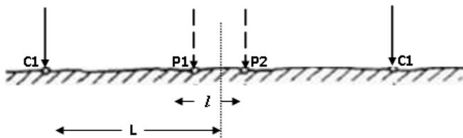
**Fig 2. The symmetrical Schlumberger array**
