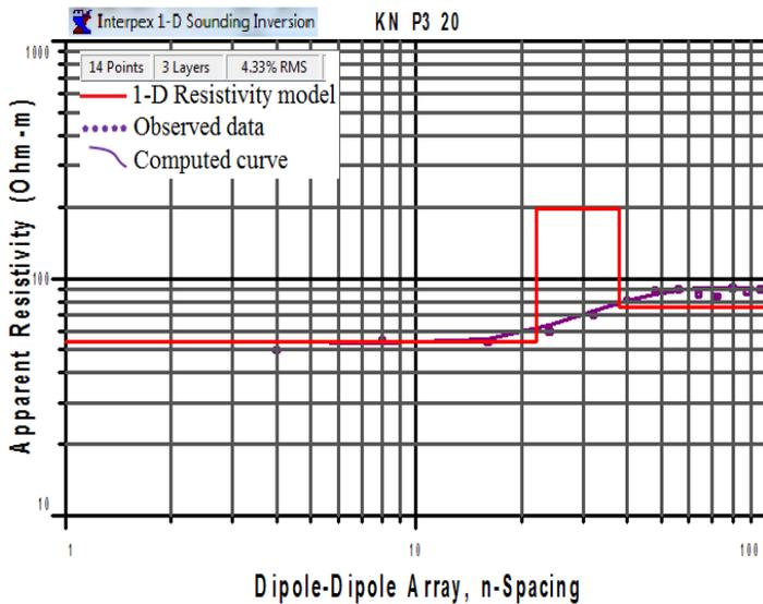
**Fig. 20** Iterated field curve and the apparent resistivity model of VES conducted at 200 m from the beginning of profile 3, Kanshegu Community(KN P3 20).
