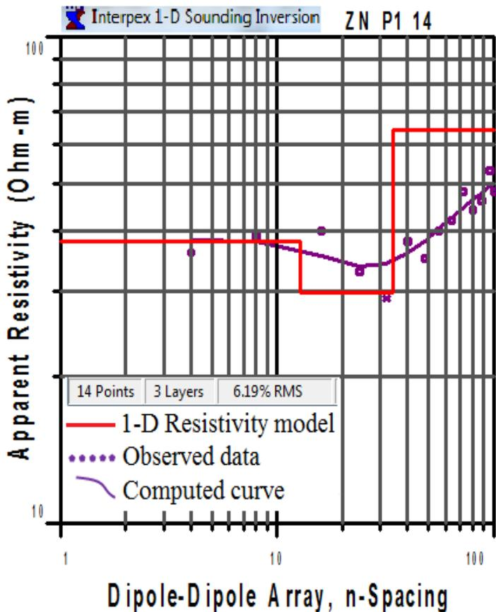
Fig. 11 Iterated field curve and the apparent resistivity model of VES conducted at 140 m from the beginning of profile 1, Zantele Community(ZN P1 14).
