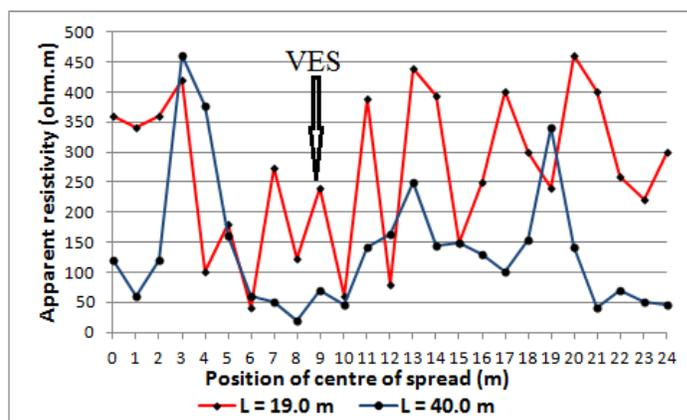
Fig. A1 Schlumberger resistivity profiles, showing apparent resistivity as a function of position of centre of spread for two values of electrode separation, Nyengbalo Community.
