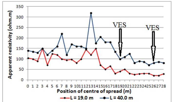
Fig. A12 Schlumberger resistivity profiles, showing apparent resistivity as a function of position of centre of spread for two values of electrode separation, Kanshegu Community.
