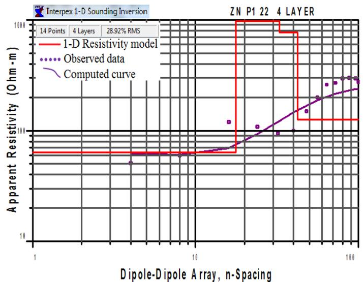
Fig. 13 Iterated field curve and the apparent resistivity model of VES conducted at 220 m from the beginning of profile 1, Zantele Community (ZN P1 22). [4 layer modeling]
