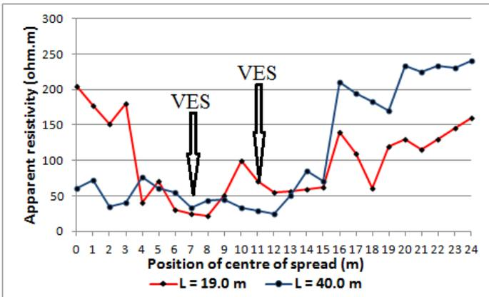
Fig. A2 Schlumberger resistivity profiles, showing apparent resistivity as a function of position of centre of spread for two values of electrode separation, Nyengbalo Community.
