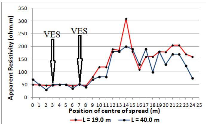
Fig. A9 Schlumberger resistivity profiles, showing apparent resistivity as a function of position of centre of spread for two values of electrode separation, Zantele Community.
