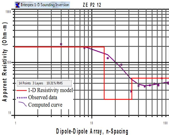
Fig. 10 Iterated field curve and the apparent resistivity model of VES conducted at 120 m from the beginning of profile 2, Zei Community(ZE P2 12).
