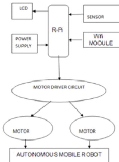
**Fig 1.** Block diagram
