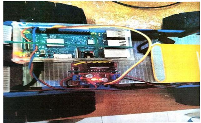
**Fig. 2.** Development of Autonomous Mobile robot with R-Pi
