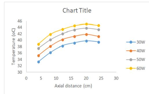
**Fig-3:** Surface temperature of the vertical cylinder along axial distance for without vibrations in the nanofluid.
