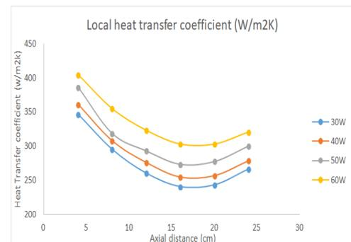
**Fig-4:** Variation of heat transfer coefficient with axial distance various heat input
