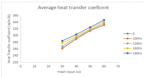
**Fig-11:** Variation of Average heat transfer coefficient with heat input
