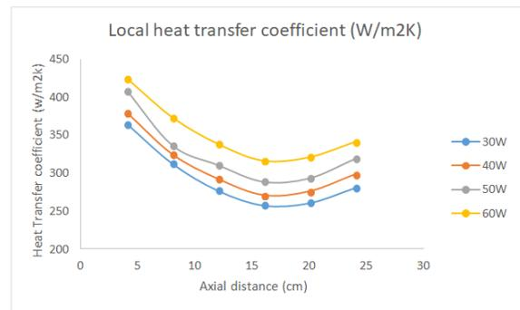
**Fig-8:** Variation of heat transfer coefficient with axial distance various heat input with vibration effect
