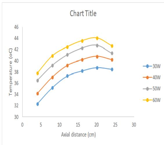
**Fig-7:** Surface temperature of the vertical cylinder along axial distance for with vibrations in the base fluid.
