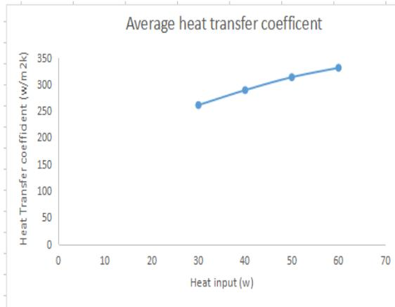
**Fig-6:** Variation of heat transfer coefficient with heat input
