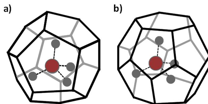
**Fig 1:** Structure 1 -Dodecahedral and Tetra decahedral water cages with CH<sub>4</sub> as guest molecule
