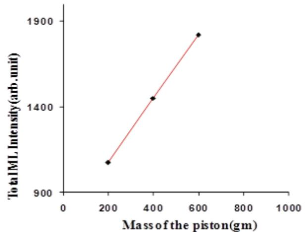
**Figure 7** The total ML intensity initially increases linearly with increasing mass of the piston
