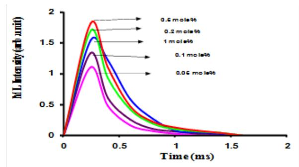
Figure 3 The ML intensity of the gamma irradiated rare earth doped phosphate based phosphors
