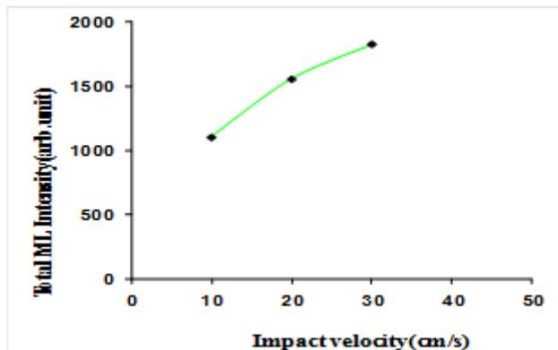
**Figure 5** The total ML intensity increases linearly with increasing impact velocity of the piston
