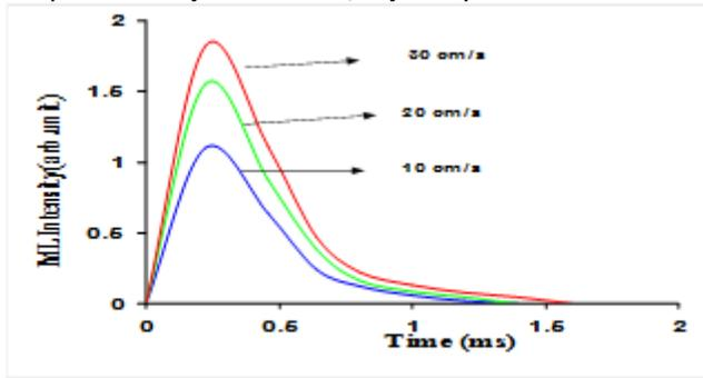
**Figure 4** ML intensity increases with increasing impact velocity of the piston
