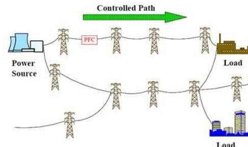
Fig3. Power flow along the controlled path.
