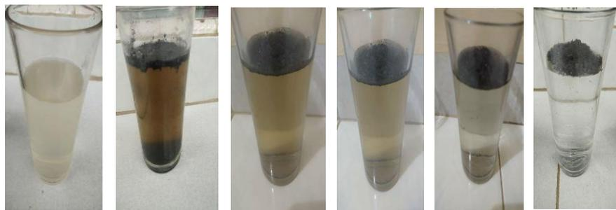
**Fig 2.** The process of activation and testing of actuary carbon samples in turbid water with a contact time of 2 hours, 4 hours, 6 hours, 8 hours and 10 hours. **Sources: Primary figure**
