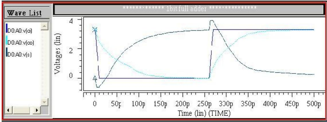
Figure 2- Simulation results of 1-bit FA.
