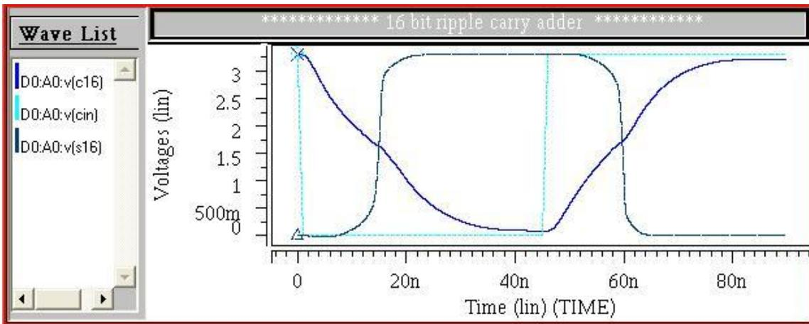
Figure 4- Simulation results of 16-bit RCA .
