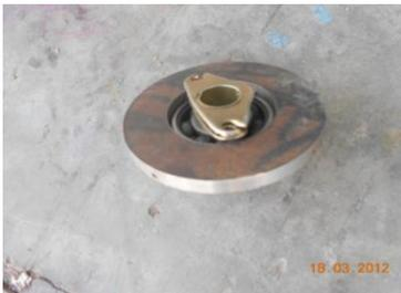
Figure 2.3 Guide Plate with Lever and bearing
