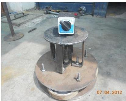
Figure 2.4 Front View of Lock Plate with magnet for attachment and deattachment of plate into machine
