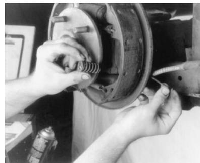
Figure 1.2 Attachment of Lock Plate (Manual)
